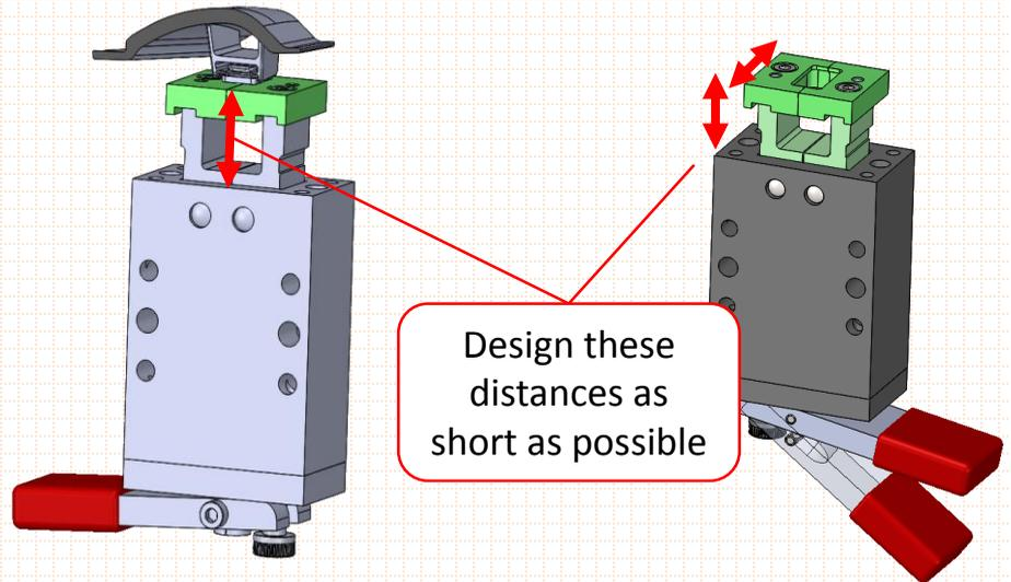
11) In general it is recommended to use Clip Buddy versions with jaw end pieces included (CB3B, CB4A, CB4B, CB5B, CB5C) whenever possible to avoid the need to fabricate, attach, and adjust jaw end pieces.
