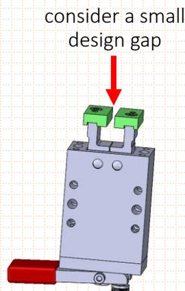
15) For machining assembled units, it is recommended to align to 2 side dowel holes and clamp the jaws across the sides for added rigidity. (for all versions, with or without jaw end pieces)
